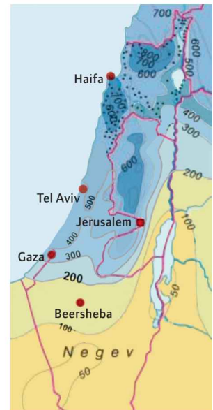
Mean annual rainfall in 100-millimeter annual precipitation isohyets, September 1931–September 1976. ATLAS OF ISRAEL
