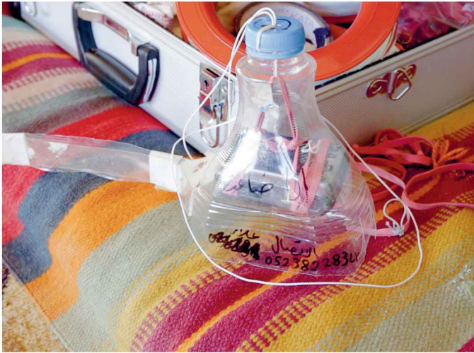
Kite kit. The camera is attached by rubber bands that keep pressing the photo button. The water bottle protects the camera at landing or if it falls. The telephone number is provided in case the camera gets lost. ALINA SCHMUCH, JAN KIESSWETTER
